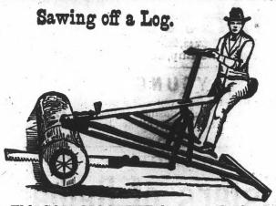
This SAW MACHINE is a wonderful invention. The weight of the man who is sawing does half of the work. It saws logs of any size, and will saw off a 2 foot log in 2 minutes. Circulars free. Address, Wm. GILES, 696 W. 6th St., Cincinnati, Ohio.
