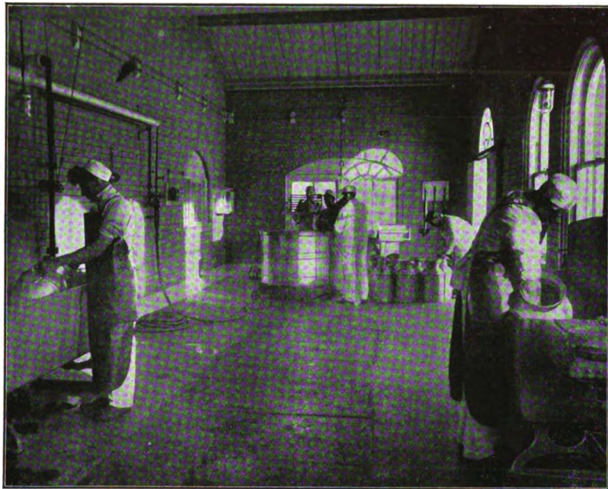
Receiving and Weighing the Milk. Cleansing the Cans With Live Steam Before They Are Returned to the Farmer. A Room Into Which Fresh Air and Sunshine Have Free Access
