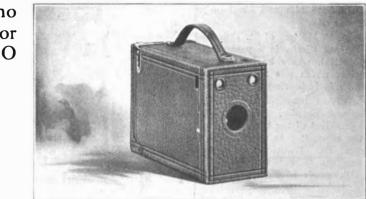
Capacity-12 films without reloading. Size of Camera-24x335x554 ins. Weight-7 ozs. Shutter-Automatic with diaphr gm' Stops. Lens-Meniscus. Finder-Dou-ble, specially treated for bril-liancy.
