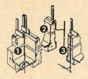
To ground a system, the conductor might be (1) carried down along wall to a rod beneath floor slab, (2) brought on outside to grade-level trench and then out 2-ft. to ground rod or (3) coursed down inside the wall.
