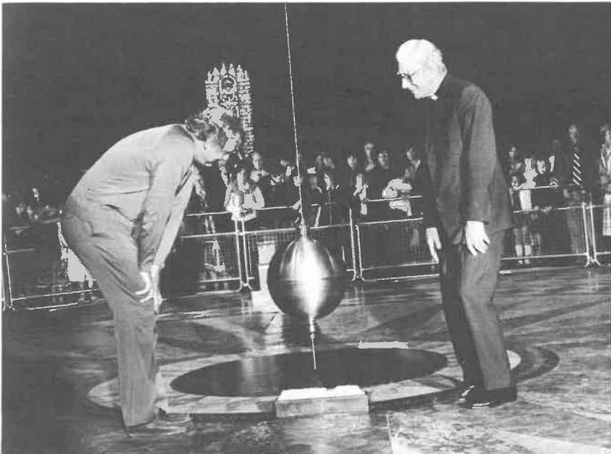
The Rev. Canon John Collins of St. Paul's Cathedral, London, and Professor Michael Pentz, dean of the Open University, witness proof of the world's rotation during a recent experiment at the cathedral. A 268" pendulum with a 150 pound brass ball was suspended from the historic dome in a reenactment of a famous experiment conducted by French scientist Jean Bernard Leon Foucault in 1851. The pendulum on a fixed pivot and a tip on the end of the ball progressively knocked down a wall of sand as the line moved around at 17 degrees an hour.
