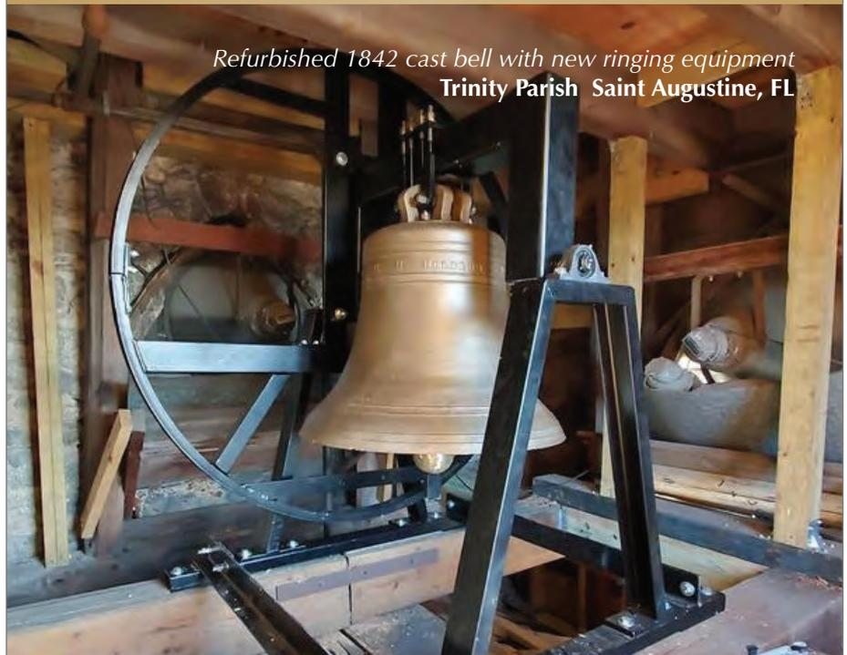
*Refurbished 1842 cast bell with new ringing equipment
